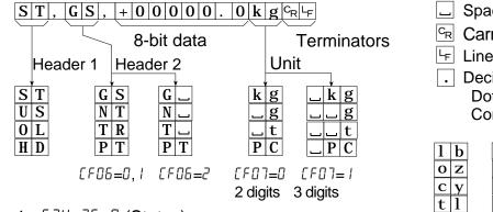
\_\_ Space code(20h)  $C_{\mathbb{R}}$  Carriage return(0Dh) Line feed(0Ah) • Decimal point : Dot(2Eh) or Comma(2Ch)
