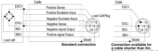
a cable shorter than 5m. (Recommended wire cross- sectional area: 0.5 mm<sup>2</sup> or greater)
