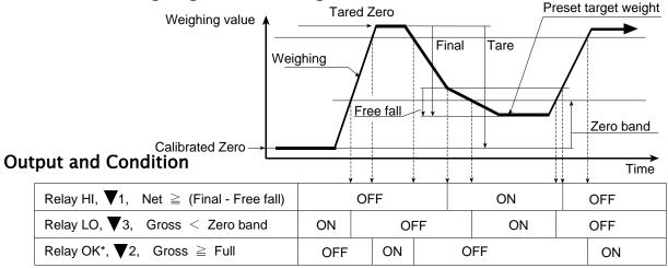
\* Relay OK output can be changed to OVER or UNDER by setting F24.
