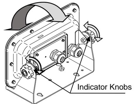
3. When using the display stand/wall-mount bracket as a wall-mount bracket, screw the stand part into a flat wall surface (screws not included). For details on installation dimensions, refer to "[11.2. Dimensions.](#)"
