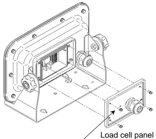
3. Loosen the lock of the cable clamp connecting to the load cell panel, and pass the load cell cable through. Fit the rubber packing in the load cell cable.
