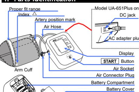
Note: Model UA-611Plus doesn't have the DC jack for AC adapter. The DC jack is located on the rear of the model, UA-651Plus only. The AC adapter is an optional accessory. (sold separately)
