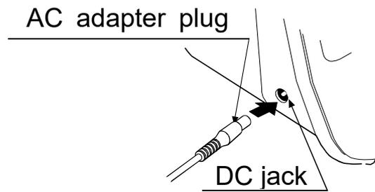
Note: The device is operated using the battery when the power is not supplied to the main body from the AC adapter.
