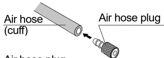
3. Connect the air hose plug of the cuff to the air hose socket of the main body.
