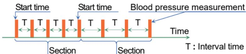
S-BPM **waiting mode** is a state that blood pressure is not being measured during the interval time and between the last "1 scope" and next "1 scope".
