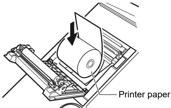
6. With the end of the paper at the top and protruding out, secure the printer paper by closing the printer cover until you hear a click. If the cover is not completely closed, a paper jam may occur.
