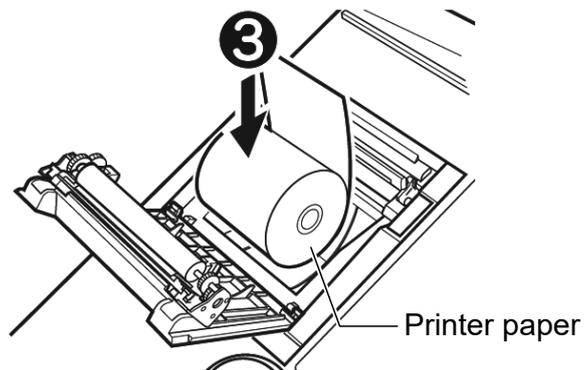
3. With the end of the paper at the top and protruding out, secure the printer paper by closing the printer cover until you hear a click. If the cover is not completely closed, a paper jam may occur.
