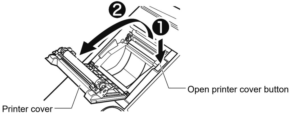
2. Install the printer paper in the way shown in the illustration below.
