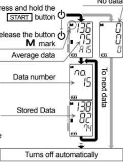
Note: If you press the [START] button while recalling data, the device turns off.
