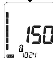
5. When the measurement is complete, the systolic and diastolic pressure readings and pulse rate are displayed. The cuff exhausts the remaining air and deflates completely.
