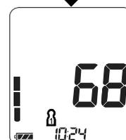
4. When inflation is complete, deflation starts automatically and ♥ (heart mark) blinks, indicating that the measurement is in progress. Once the pulse is detected, the mark blinks with each pulse beat.
