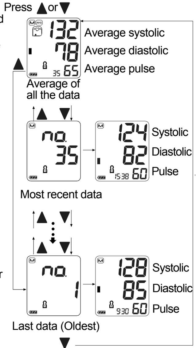
4. Press the **SET** button to change the user and display the memory display for that user.
