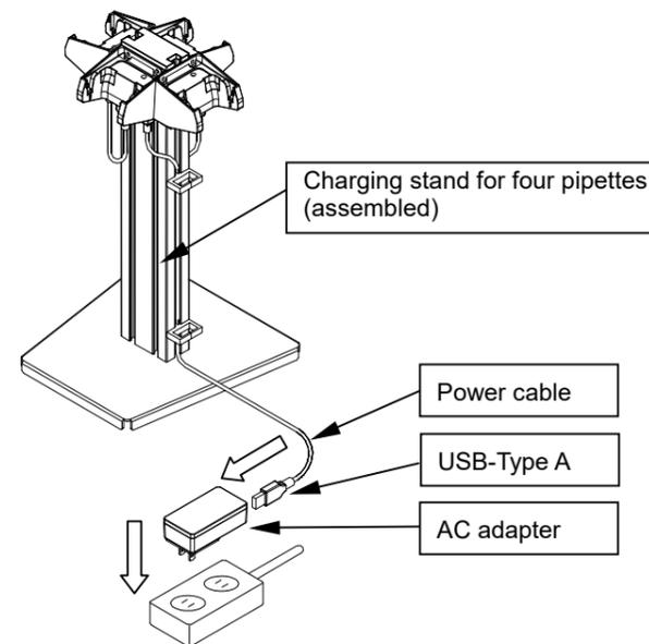
4. Hook the PA/PB onto the charging sections to start charging. Once charging starts, the battery indicator at the bottom left of the PA/PB display will blink as shown in the figure on the right.
