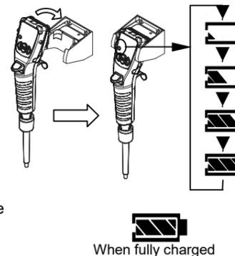
5. Charging is complete when the PA/PB battery indicator is fully lit.
