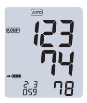
After the resting time has elapsed, multiple measurements are made at specified time intervals.
