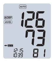
After the measurement is completed, the average value is displayed.
