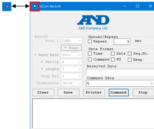
Step 4 When the stability mark of a balance is displayed and the [Print] key of a balance is pressed, the current data is transmitted to a computer.
