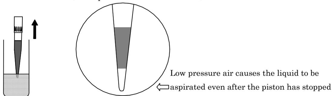
(3) Use a tip with a large tip end diameter (cut off the end of the tip, etc.)
