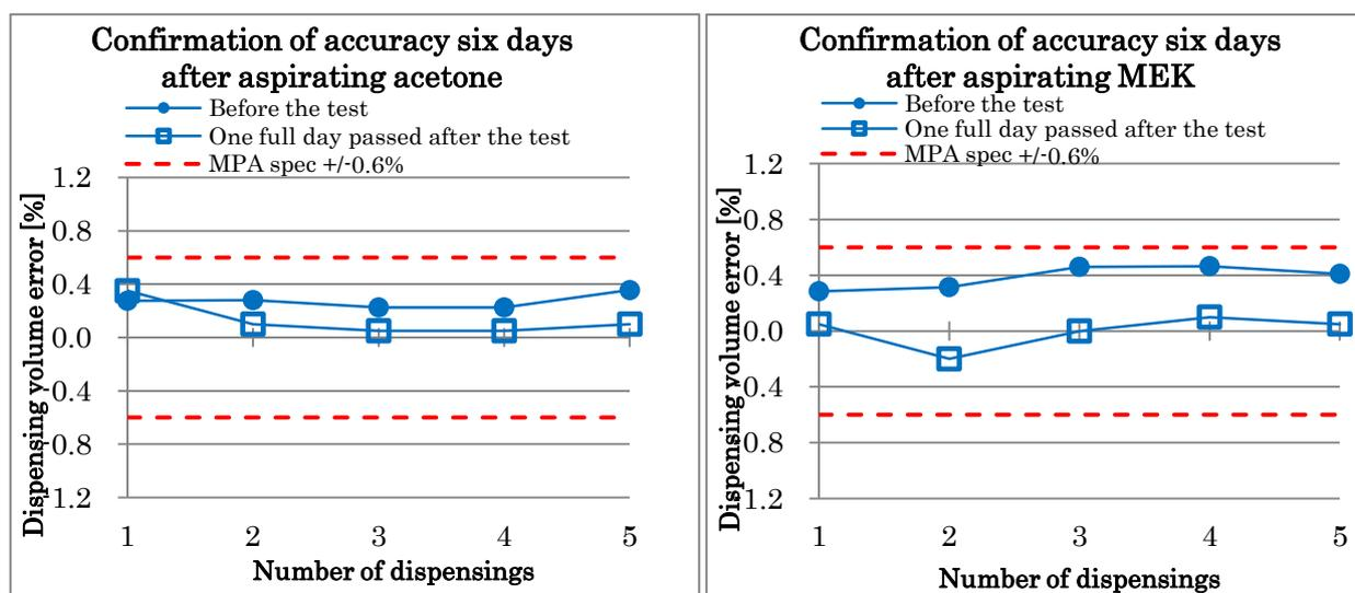
\* Accuracy was tested one day after discharging the solvents from inside the tip
