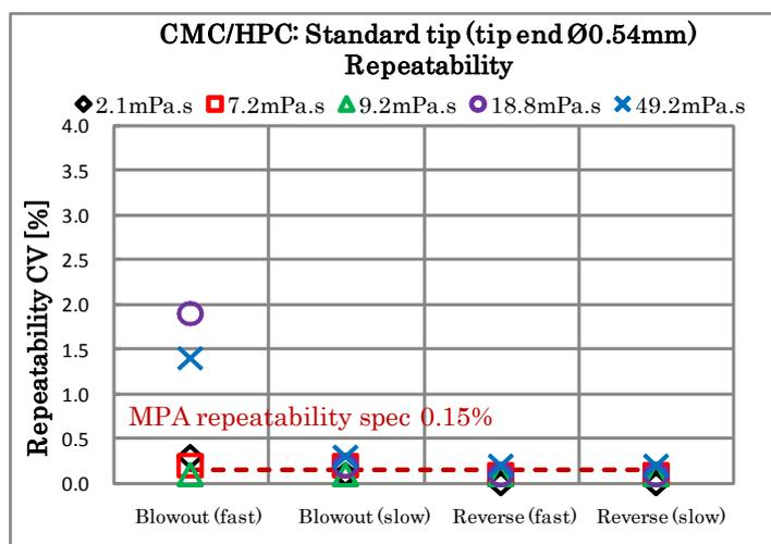
When viscosity levels reach around 50mPa.s, air is discharged before the liquid and the amount dispensed becomes less than the amount specified.
