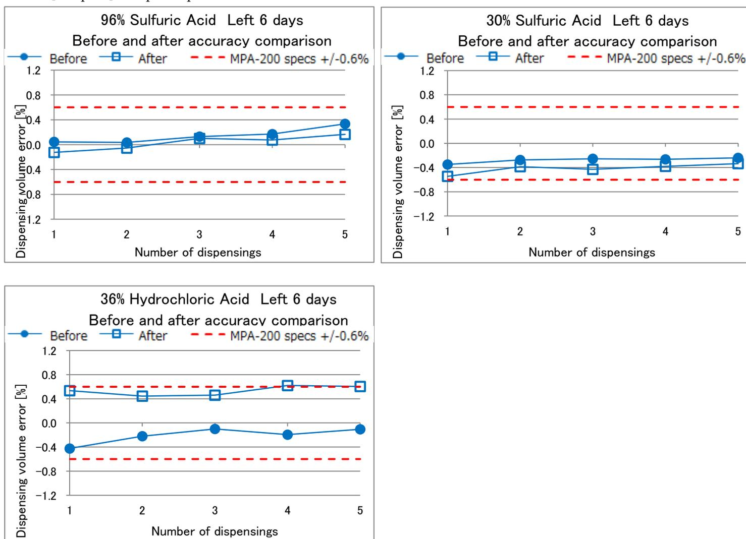
For the sulfuric acid (96%, 30%) there was no observed deterioration of the main body or effect on the accuracy of measurement.
