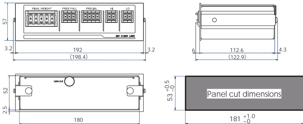
1. The dimensions of OP-05 and OP-06 are almost identical, while the panel cut dimensions are exactly the same. It is possible to easily shuffle between OP-05 and OP-06 installed on the instrumentation board.
