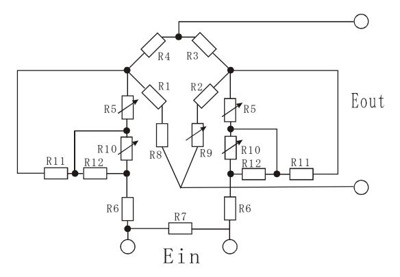
Figure 2.13. Load cell circuit
