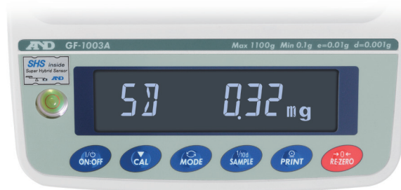
Standard deviation calculated using ECL
