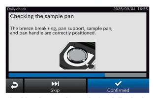
Checking the sample pan during daily checks
