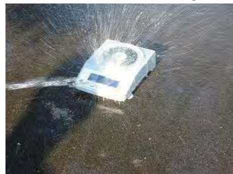
Water jet directed to the front of the test sample
