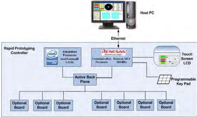
**Figure 2. Hardware Architecture of the Rapid Prototyping Controller**
