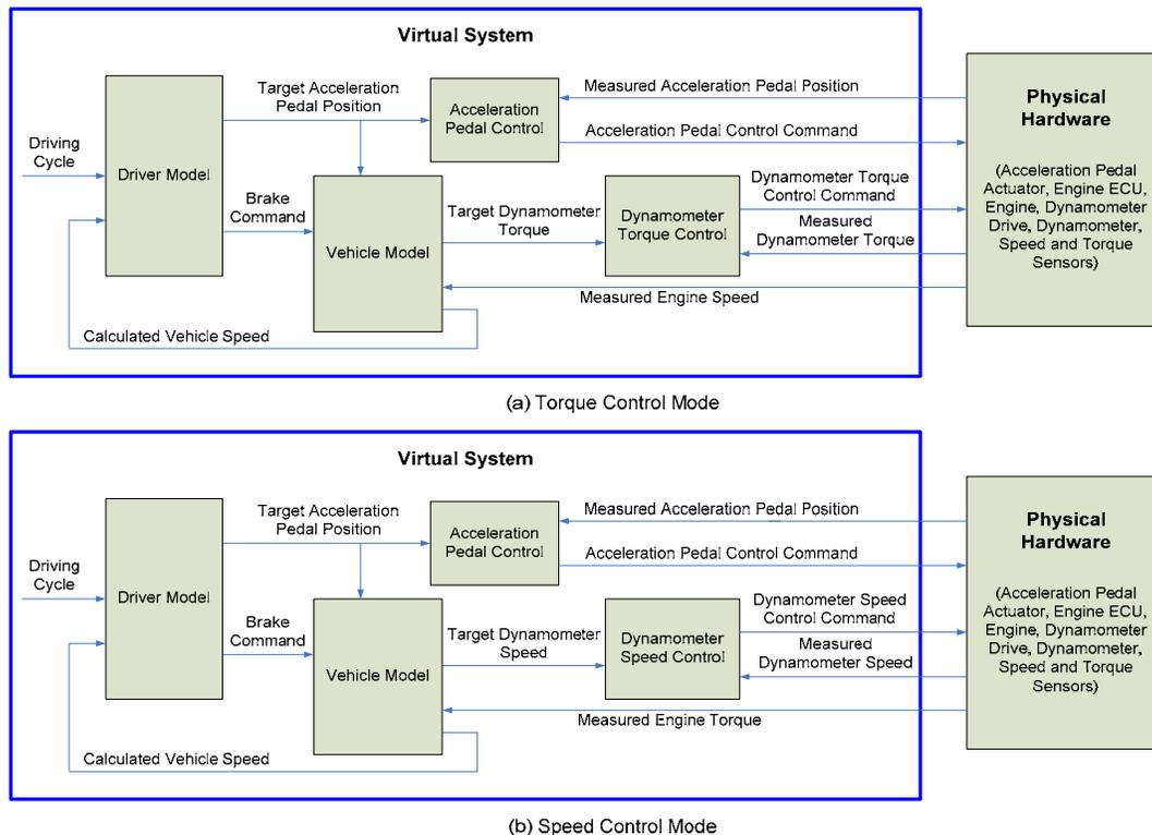
**Figure 4. Simulation and Control Model Structure**
