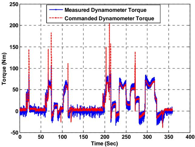
Figure 8. Commanded and Measured Dynamometer Torque
