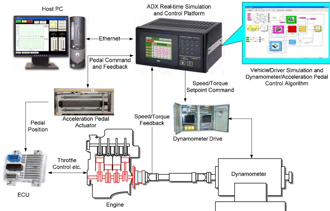
**Figure 2. Overall Structure of the EIL System**
