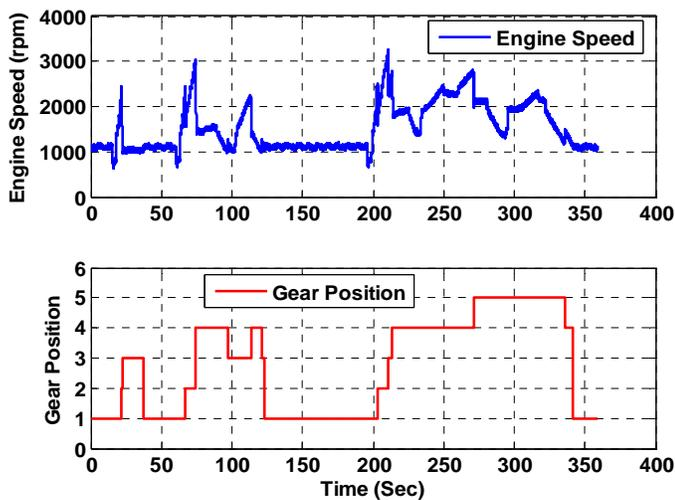
Figure 9. Engine Speed and Automatic Transmission Gear Position
