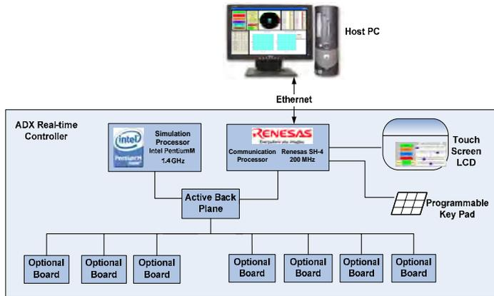
**Figure 3. Hardware Architecture of the ADX Real-time Controller**
