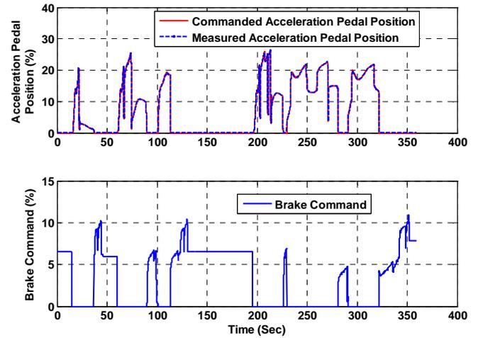
Figure 10. Acceleration Pedal Control and Brake Command
