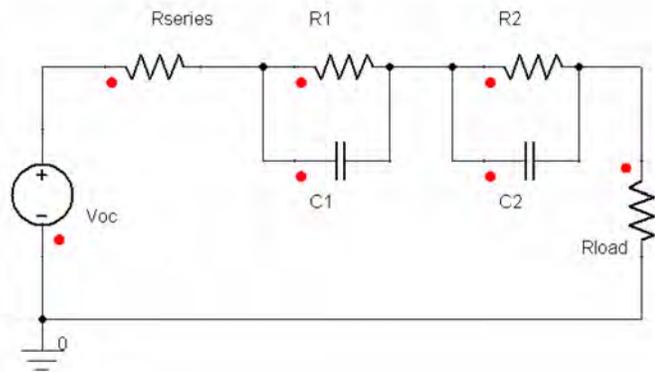
Fig. 1. A battery equivalent circuit model.
