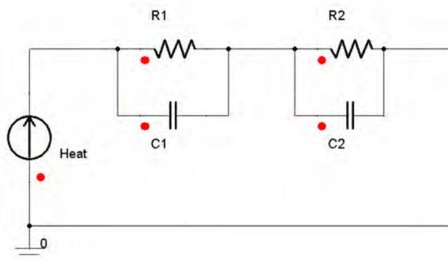
Fig. 2. An LTI model for battery thermal system.
